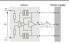
In the same way as for current sensors, this secondary current I can be then passed through a measuring resistance R<sub>m</sub>. The measuring voltage  $V_m$  at the terminals of this measuring resistance  $\boldsymbol{R}_{\!_{m}}$  is therefore also exactly proportional to the primary voltage U<sub>p</sub>. The electrical supply to the sensor is also insulated from the primary voltage.
