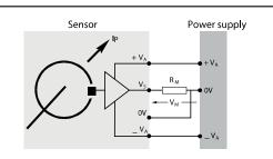
The secondary output voltage  $V_s$  is therefore directly proportional to the primary current. It is an exact replica of the primary current, generally with a value of 4 V for a nominal current IPN.
