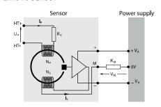
Principle diagram of a calibrated EM010 sensor
