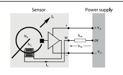
The secondary output current I<sub>s</sub> is therefore exactly proportional to the primary current at any moment. It is an exact replica of the primary current multiplied by the number of turns  $N_p/N_s$ . This secondary current I<sub>s</sub> can be passed through a measuring resistance R<sub>M</sub>. The measuring voltage V<sub>M</sub> at the terminals of this measuring resistance R<sub>M</sub> is therefore also exactly proportional to the primary current I,
