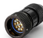
Cable-connecting socket, long housing, 10 pole to VG96934 version J for connection and interconnection cables, available with 5-coding layers and solder terminals up to AWG20
