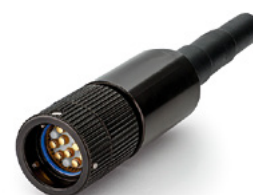
Cable-connecting plug with rubber sleeve, 10 pole to VG96934 version J for connection and interconnection cables, available with 5-coding layers and solder terminals up to AWG20
