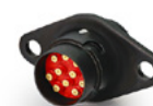
Flange socket, 10 pole to VG96934 version J for housing installation, available with 5-coding layers and solder and PCB connection
