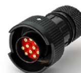
Cable-connecting socket with step protection, 10 pole to VG96934 version J for connection and interconnection cables, available with 5-coding layers and solder terminals up to AWG20
