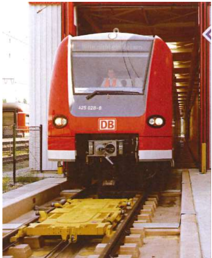
Train washing plant (PINPOSITON 300)
